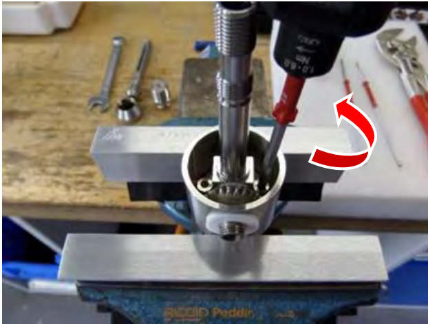
Loosen holding screw (2.14)
