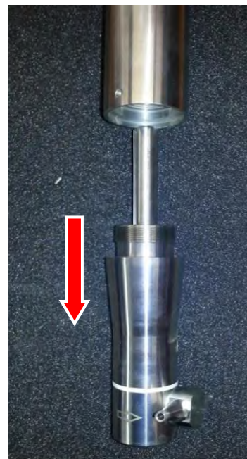
Pull out head AG with adapter (2)
