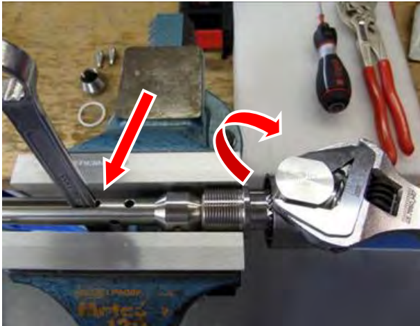
Tighten the Nozzle Carrier (3.1)
