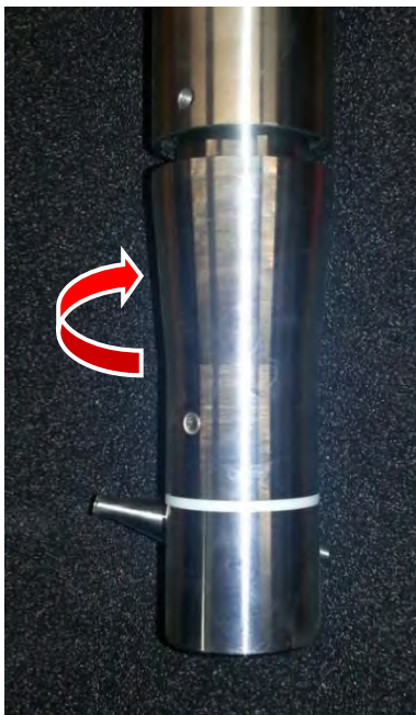
Unscrew head AG with adapter (2)
