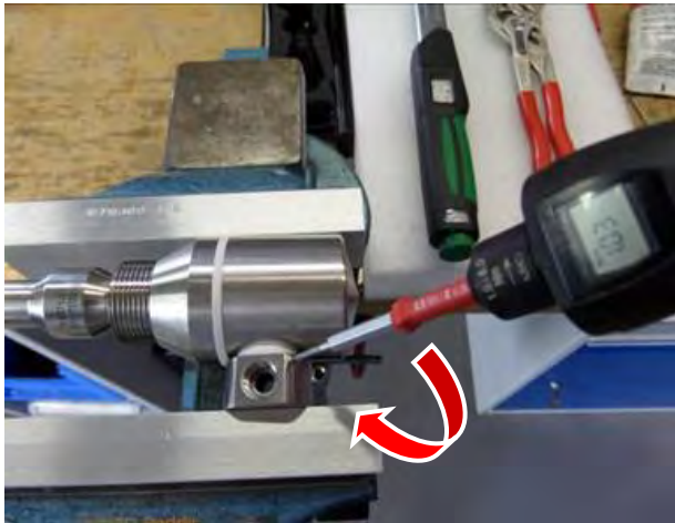
Tighten the Set Screw (3.2)
