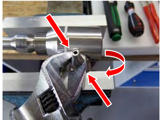
Tighten the Nozzle (3.5)
