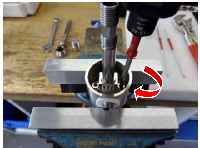
Tighten the Holding Screw (2.14)
