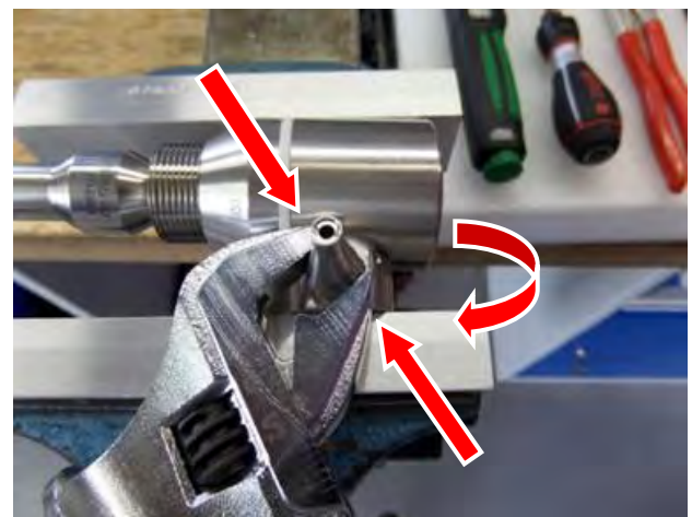
Tighten the Nozzle (3.5)
