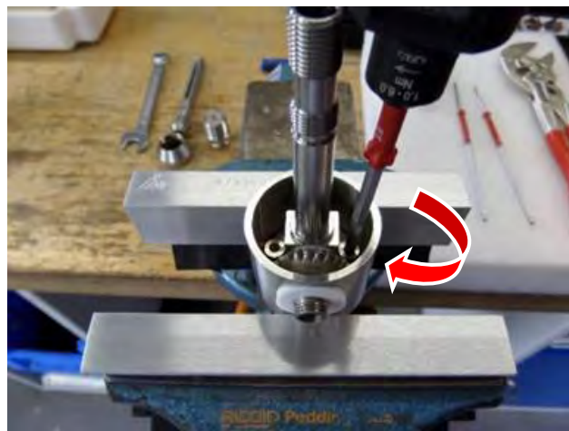
Tighten the Holding Screw (2.14)
