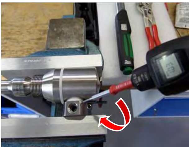
Tighten the Set Screw (3.2)
