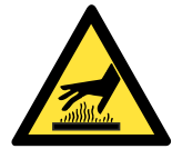
Warning of a hot surface
