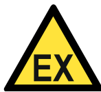
Warning of a potentially explosive atmosphere
