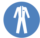
Wear protective work clothing
