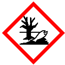
Warning about substances that are a water hazard
