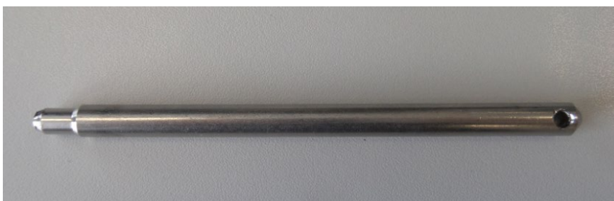
Figure 7.4-3: Assembly tool for wire locking pin
