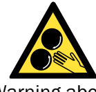
Warning about trapping/entanglement hazard
