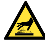
Warning of a hot surface
