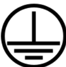
Protective grounding connection required
