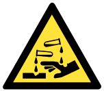
Warning of corrosive substances
