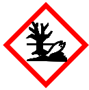
Warning of substances that pose a water hazard
