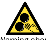
Warning about trapping/entanglement hazard
