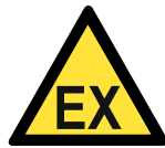
Warning of a potentially explosive atmosphere
