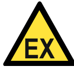
Warning about explosive atmosphere
