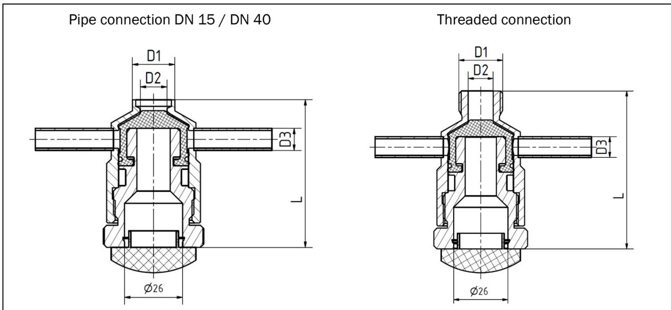
Fig. 4-5: Pipe connection variants, thread for Standard Vario
