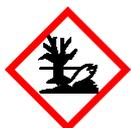
Warning about substances which are a water hazard is indicated by this symbol.
