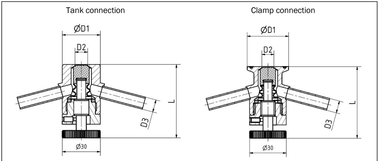
Fig. 4-2: Tank connection variants, clamp for compact EHEDG
