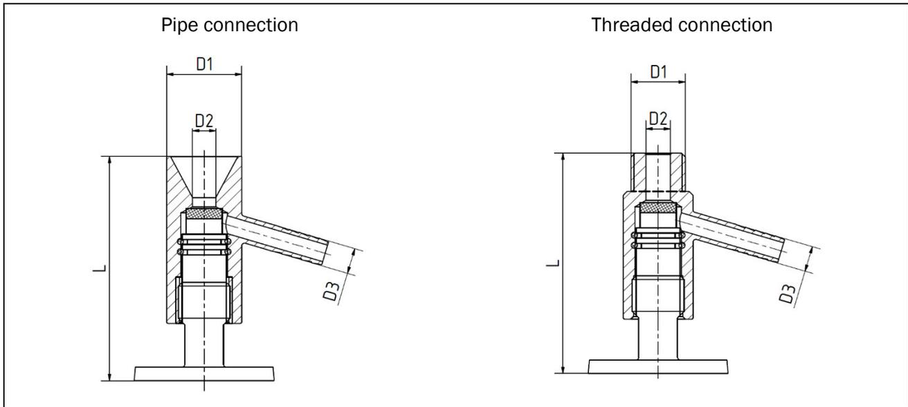
Fig. 4-4: Pipe connection variants, thread for Standard ECO
