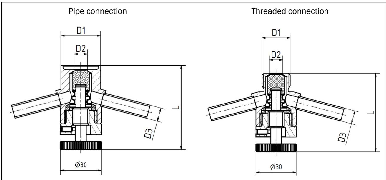
Fig. 4-1: Pipe connection variants, thread for compact EHEDG
