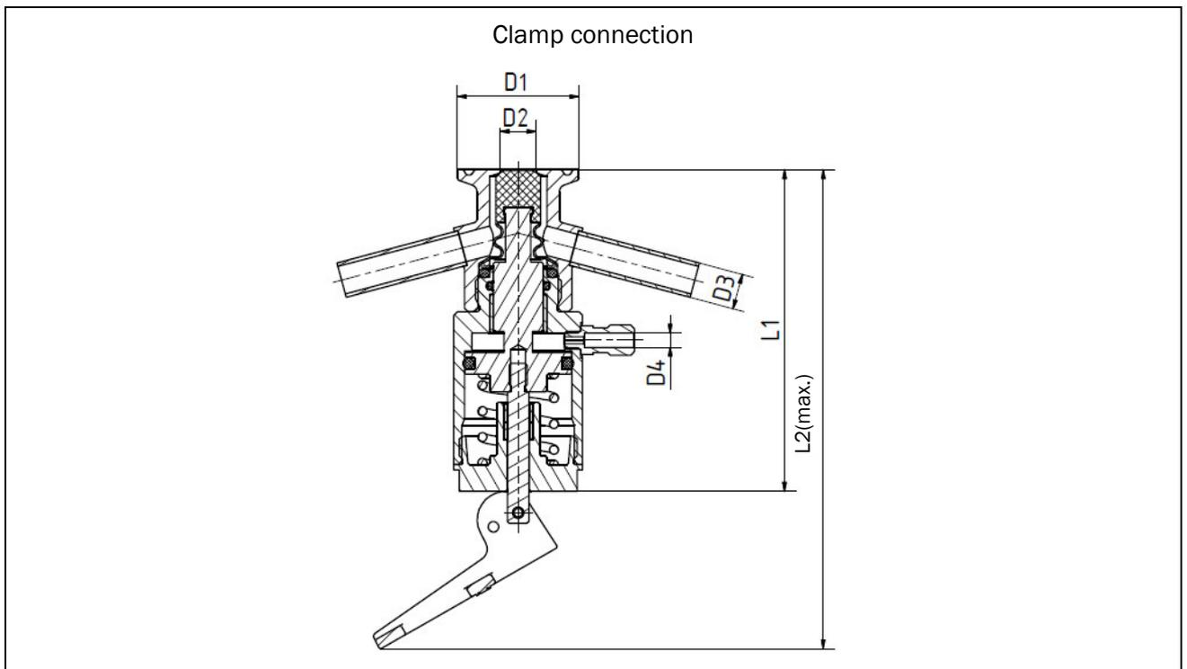
Fig. 4-3: Connection variant clamp for PNV compact air
