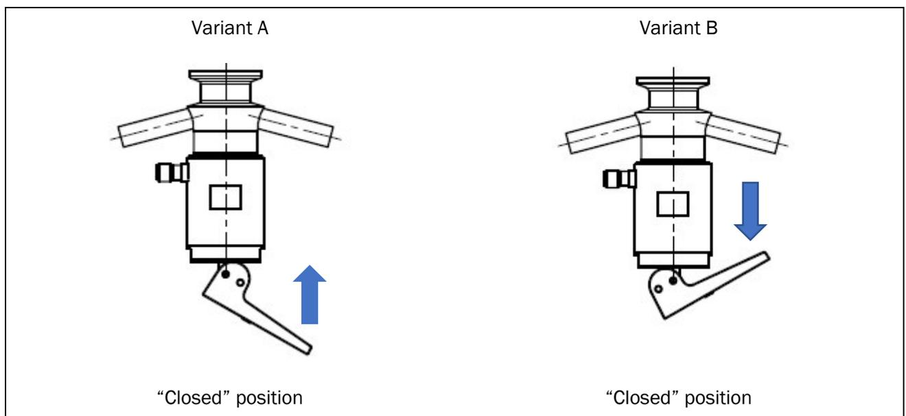
Fig. 6-2: Conversion of variant A to variant B
