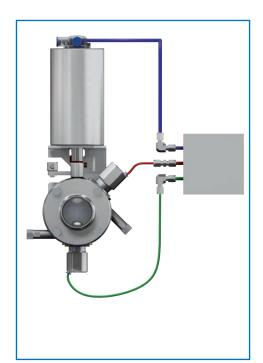
If only one control air line is in use, the two auxiliary valves open for flushing and draining when the flaps of the butterfly valve are closed.
